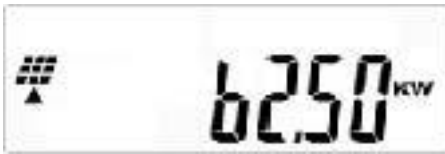
Fig. 7-4 - 11 Display Q - String B output power
