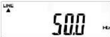
Fig. 7-4 - 13 Display S - Frequency of the photovoltaic solar inverter output voltage
