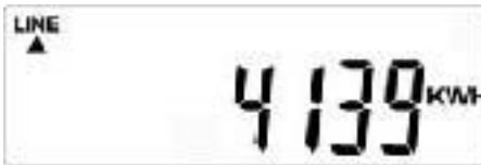
Fig. 7-4 - 1 Display G - Total feed power
