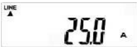
Fig. 7-4 - 14 Display T - Output current of the photovoltaic solar inverter
