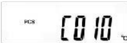
Fig. 7-4 - 2 Display H - Internal temperature of the photovoltaic solar inverter in °C
