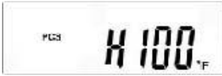
Fig. 7-4 – 5 Display K - Temperature of cooling element in °F
