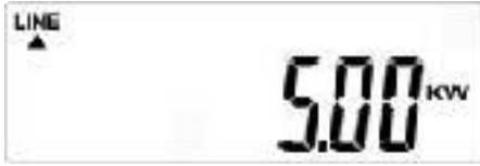
Fig. 7-4 - 15 Display U - Current feed power
