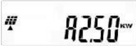
Fig. 7-4 - 10 Display P - String A output power
