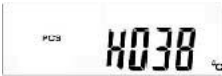
Fig. 7-4 - 3 Display I - Temperature of cooling element in °C
