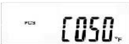
Fig. 7-4 - 4 Display J - Internal temperature of the photovoltaic solar inverter in °F
