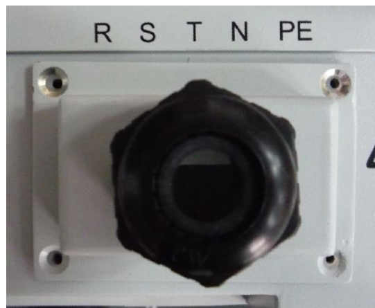
Fig.11 - Terminal board for AC cables connections
