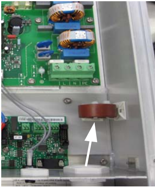
Figure 14: Insert AC leads into the connection area
