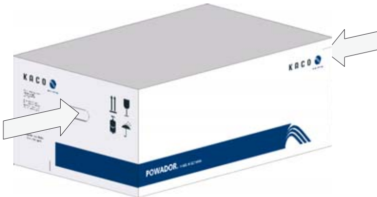
Figure 7: Transportation of the inverter
