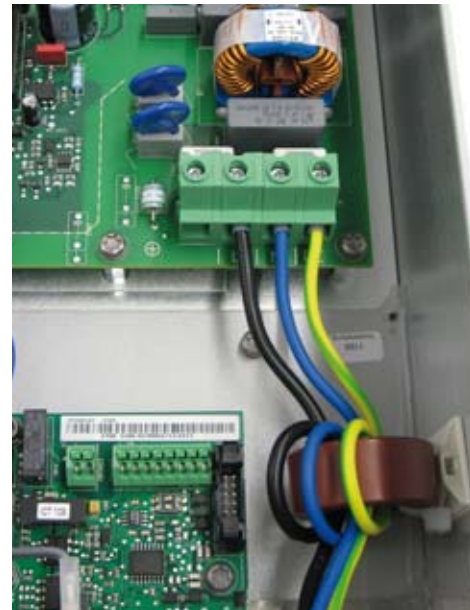
Figure 15: AC leads wound around the ferrite cores
